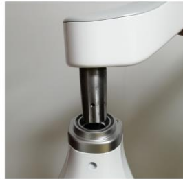
2. Connect the plug of the rotational arm and the main frame
